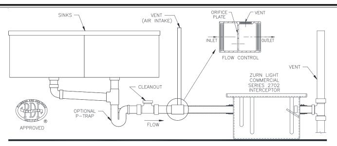
Zurn Light Commercial Series Grease Interceptors GT2702 consist of a interceptor rated at ( ) gpm and a properly sized flow control fitting.
