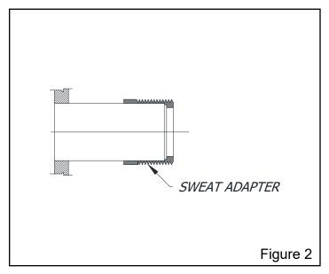
2. Slide threaded adapter onto supply pipe until shoulder stops on end of pipe. Then sweat-solder the adapter to water supply pipe.
