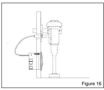
Feed motor cable from actuator to enclosure. Connect the motor cable from actuator to the large three wire motor cable connector exiting the backside of enclosure.
