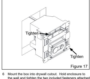
the wall and tighten the two included fasteners attached to blue box.
