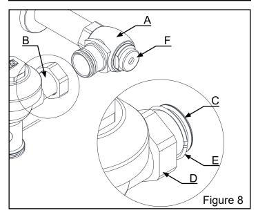
Prior to attaching flush valve (B) to control (A) inspect and verify that the O-ring seal is located within the O-ring groove (C) at the tailpiece. Ensure the locking nut (D) and locking snap ring (E) are also present on the tailpiece. Lubricate O-ring with water if necessary and insert flush valve tailpiece into the control stop valve. Tighten locking nut (D) using a smooth jawed wrench.
