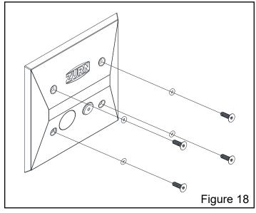
7. Apply light pressure to sensor faceplate while assembling to compress gaskets while tightening fasteners with supplied allen wrench.
