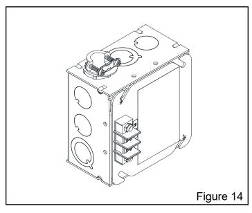
Loosen cover retaining screw with Phillips head screw driver to remove cover from HW6 enclosure. Feed power cord into enclosure box through wire clamp (not provided). Tighten screws clockwise on wire clamp to secure power cable in place.
