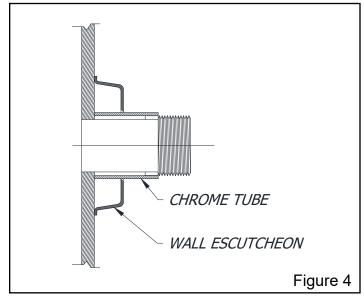
4. Slide wall escutcheon over chrome tube and slide both chrome tube and wall escutcheon over supply pipe pushing the wall escutcheon all the way to the wall.
