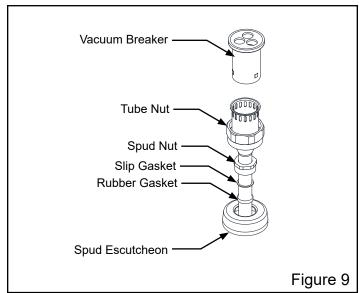
Slide the tube nut, spud nut, slip gasket, rubber gasket and spud escutcheon over the vacuum breaker tube and insert tube into fixture spud. Hand tighten tube nut to valve body and hand tighten spud nut onto fixture spud. Adjust the valve assembly for plumb. Tighten fixture spud nut, vacuum breaker tube nut and lock nut with a wrench.
