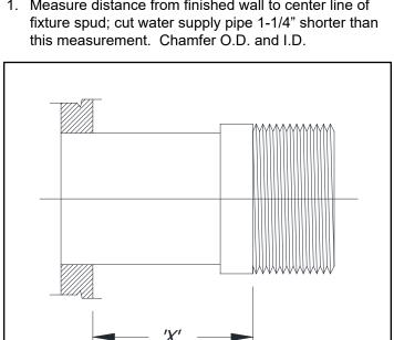
3. Measure from finished wall to first thread of adapter for length of chrome tube. Cut chrome tube this length 'x'.
