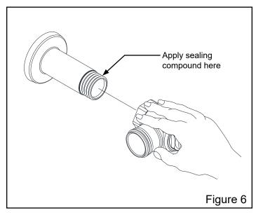
Install control stop assembly by threading it onto water supply pipe and tightening with a smooth jawed wrench. Apply thread sealing compound or pipe tape to male NPT thread on sweat solder adapter only.
