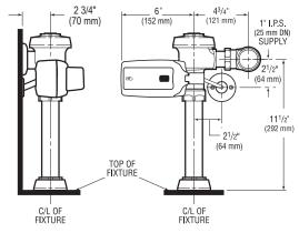
**NOTE**: All vitreous china dimensions shown in these drawings are nominal. Dimensions can vary within the tolerances established in the governing ASME A112.19.2/CSA B45.1 standard. Please take this into consideration when planning rough-in and plumbing layouts.
