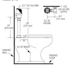
The Model 8115 valve is designed for installations where the water supply is roughed-in 24" (610 mm) above the top of the water closet. For new installations, Sloan strongly recommends the use of our Model 8111 valve which has a shorter installation height.
