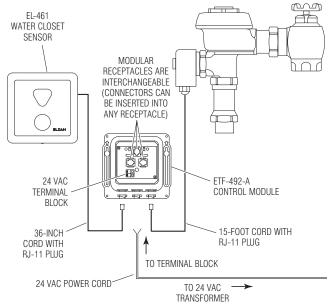
One 50 VA Transformer serves up to ten (10) OPTIMA Closet/Urinal Flushometers. Specify number of transformers required accordingly.
