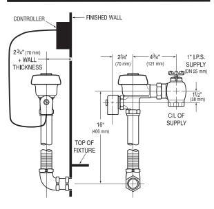
3 ¼" (83mm) LONG FLUSH TUBE FOR CONNECTION BEHIND WALL. CONNECTION THROUGH WALL NOT SUPPLIED BY SLOAN ON STAINLESS STEEL FIXTURES.
