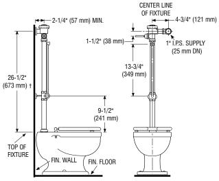
IF VALVE IS NOT PROVIDED WITH 13-1/2" (343 mm) V-600-AA VACUUM BREAKER, CUT VACUUM BREAKER TUBE TO SIZE TO MEET ROUGH-IN HEIGHT.
