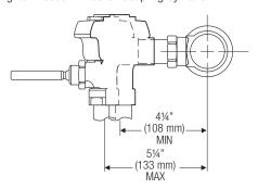
Maximum adjustment of the Sloan Adjustable Tailpiece is 1/2" (13 mm) IN or OUT from the standard 4-3/4" (121 mm) (centerline of Flushometer to centerline of Control Stop).
