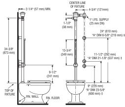
‡ DIMENSION "A" IS LENGTH OF PIPE REQUIRED TO RAISE THE SUPPLY TO THE CONTROL STOP. ELBOW FITTING SUPPLIED.
