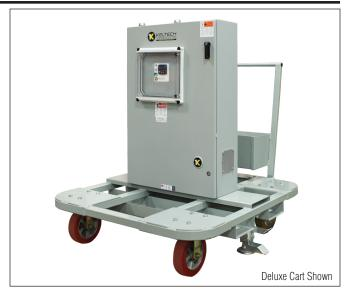
The standard cabinet enclosure is NEMA 4 rated and made from 16 gauge mild steel and powder coated with ANSI 61 gray, corrosive resistant paint. The optional NEMA 4X enclosures are for harsher environments and made from 16 gauge 304 stainless steel. The NEMA 4X enclosure can also be specified with 316 stainless steel (at additional price). Keltech Portable Heaters include tamper resistant latches with matching quarter-turn tools to inhibit unauthorized access.
