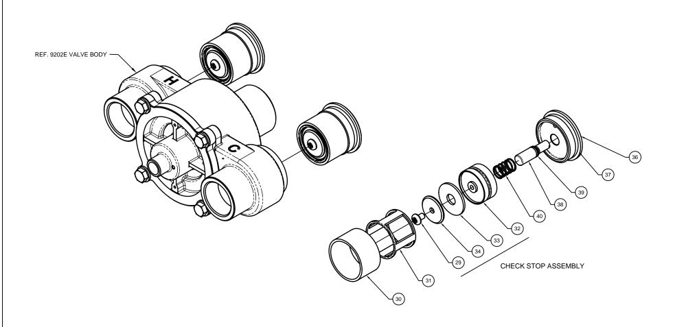
NOTE: HOT AND COLD CHECK STOPS ARE IDENTICAL. KIT INCLUDES BOTH.
