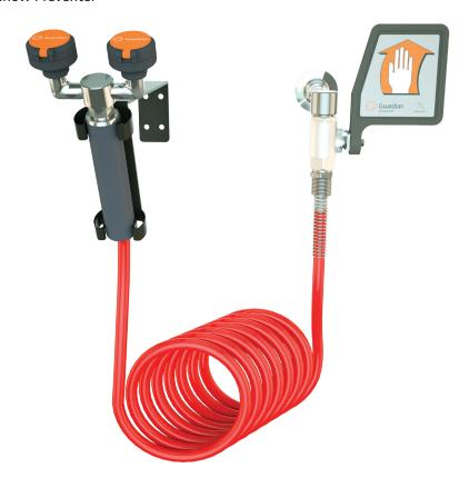
**Application:** Dual purpose eyewash/drench hose with ball valve and flag handle for wall mounting. Unit meets the provisions of ANSI Z358.1-2014 as both an eyewash and a drench hose. Unit may be left in the mounting bracket for use as a fixed eyewash, leaving user's hands free. Alternatively, unit may be removed for use as a drench hose to rinse any part of user's eyes, face or body. 12' nylon retractable hose coils to eliminate trip hazard.
