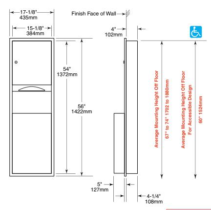
Rough Wall Opening 15-3/4" (400mm) wide 54-3/4" (1390mm) high 4" (102mm) minimum recessed depth
