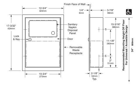
Rough Wall Opening 10-3/4" (273mm) wide 15-3/16" (386mm) high 3-15/16" 100mm) minimum recessed depth
