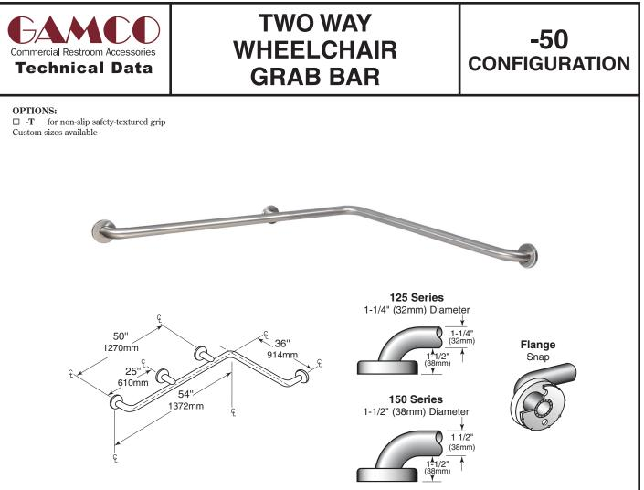
Center post needed on bars over 48" (1219mm).
