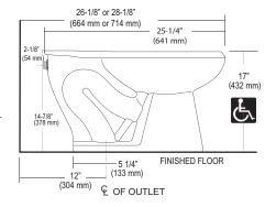
NOTE: All vitreous china dimensions shown in these drawings are nominal. Dimensions can vary within the tolerances established in the governing ASME A112.19.2/CSA B45.1 standard. Please take this into consideration when planning rough-in and plumbing layouts.
