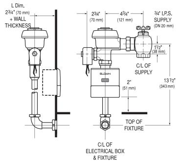
ELECTRICAL BOX INSTALLATION SENSOR LOCATION AND POSITIONING IS CRITICAL
