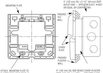
ATTACH MOUNTING PLATE TO PLASTER RING USING FOUR (4) SCREWS (SUPPLIED) 4" (102 mm) SQ. BOX DEVICE COVER (PLASTER RING) 3/4" (19 mm) HIGH — APPLETON ELECT. #8470 OR EQUAL (BY CONTRACTOR)
