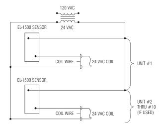
One Transformer serves up to ten (10) OPTIMA Closet/Urinal Flushometers. Specify number of transformers required accordingly.
