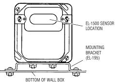
Adjust the Mounting Bracket so that the Sensor sits flush against the Cover Plate. Refer to the instructions packaged with the Flushometer for additional installation information.
