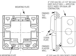
ATTACH MOUNTING PLATE TO PLASTER RING USING FOUR (4) SCREWS (SUPPLIED) 4" (102 mm) SQ. BOX DEVICE COVER (PLASTER RING) 3/4" (19 mm) HIGH — APPLETON ELECT. #8470 OR EQUAL (BY CONTRACTOR)
