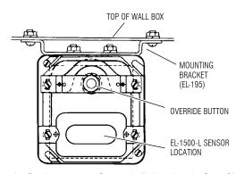
Adjust the Mounting Bracket so that the Sensor sits flush against the Cover Plate.
