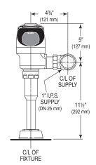
3. When the user steps away from the OPTIMA Plus Sensor, the Sensor initiates an electrical signal that operates the Solenoid. This initiates the flushing cycle to flush the fixture. The Circuit then automatically resets and is ready for the next user.
