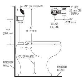
The Model 8116 valve is designed for installations where the water supply is roughed-in 27" (686 mm) above the top of the water closet.
