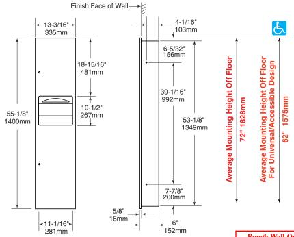
Rough Wall Opening 11-1/2" (392mm) Wide 53-5/8" (1362mm) High 5-3/8" (146mm) minimum recessed depth
