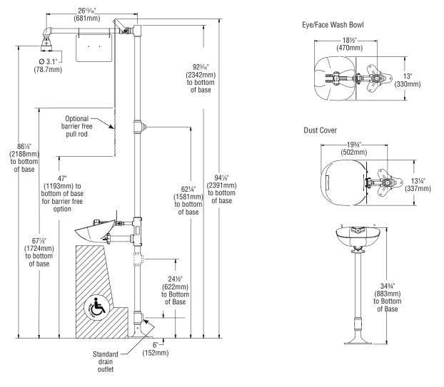
All dimensions assume standard thread engagement. Variations in manufacturing allow for  $+/-\frac{1}{3}$ "(3mm) per threaded joint. To find the tolerance of a dimension, add the number of thread joints across the length of the dimension and multiply it by  $\frac{1}{3}$ " (3mm).
