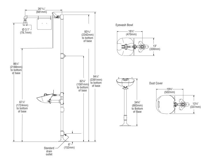
All dimensions assume standard thread engagement. Variations in manufacturing allow for  $+/- \frac{1}{3}$ "(3mm) per threaded joint. To find the tolerance of a dimension, add the number of thread joints across the length of the dimension and multiply it by  $\frac{1}{3}$ " (3mm).
