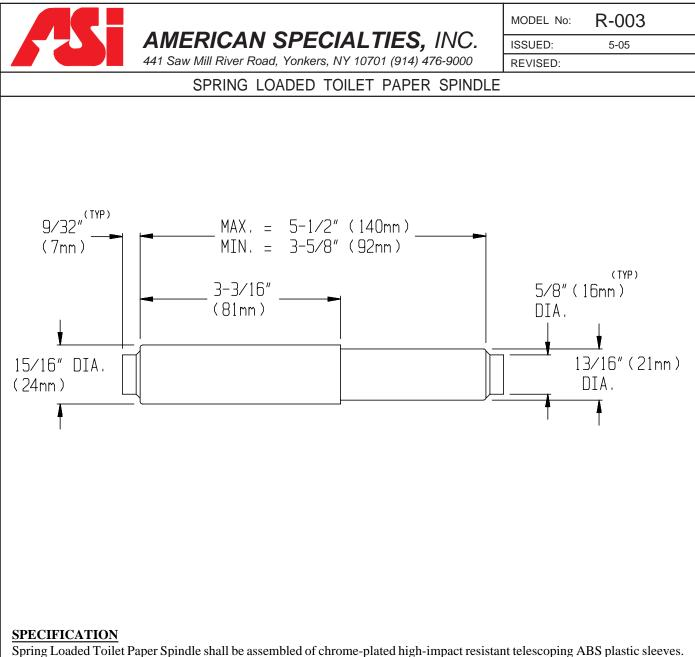
Spring Loaded Toilet Paper Spindle shall be assembled of chrome-plated high-impact resistant telescoping ABS plastic sleeves. Internal heavy duty spring shall be corrosion resistant plated steel or stainless steel. Roller shall be 5-1/2" (140mm) long to fit between the toilet paper holder posts with spring tension and have 5/8" (16mm) diameter hubs at each end to fit standard posts. Standard core toilet paper roll shall be accommodated.
